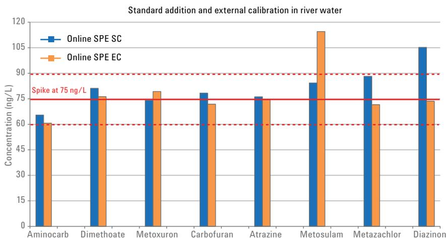
Figure 3. Comparison of the standard addition calibration to an external calibration in drinking water. A 75 ng/L amount of pesticides were spiked in river water.
